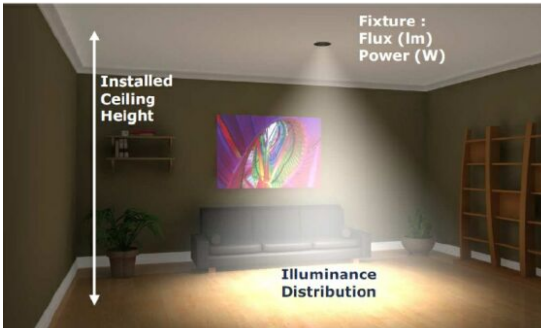
Figure 1 - Critical Characteristics for Example CFL Downlight
